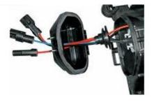
3. CONNECT INTERNAL POWER WIRES (OEM INPUT) TO VEHICLE AND SECURE BULB IN TO PLACE.
