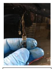
Wires connected, we recommend insulting wires with heat shrink and/or electrical tape to prevent contacts from touching.
