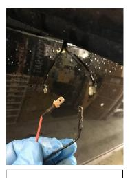
Connect the wires of the LED puddle lamps; they are non-polar meaning you can connect either wire to either on the truck.
