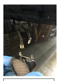
Remove the spade connectors from the factory wiring on vehicle as shown above; be sure to not let them touch.
